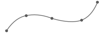
FIGURE 27 A spline curve formed with individual cubic polynomial sections between specified coordinate positions.
