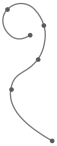
FIGURE 1 A set of six control points interpolated with piecewise continuous polynomial sections.
