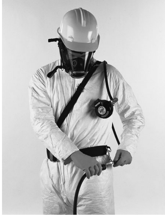
Figure 20–14 Hose fed respirator. Courtesy of Scott health and Safety.
